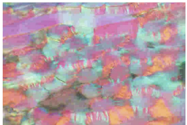
Fig. 6. Optical micrograph of cross-sectional view of carbon sample with 23 vol.% matrix content ( \times 100).
